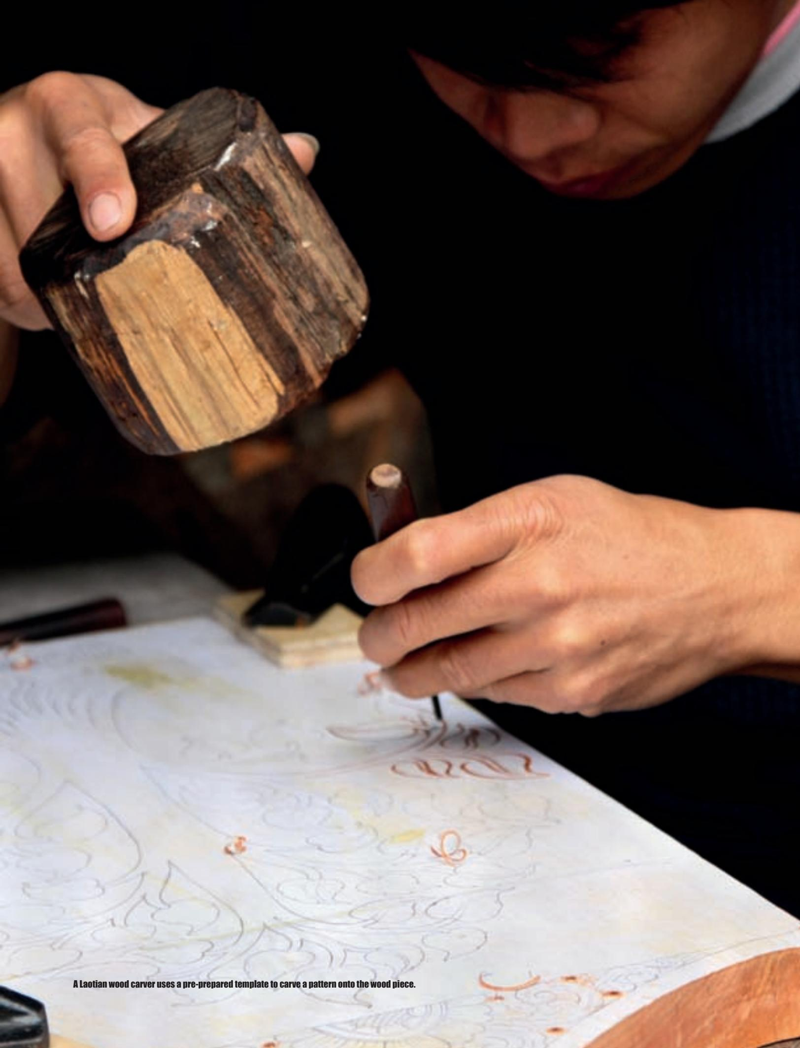
A Laotian wood carver uses a pre-prepared template to carve a pattern onto the wood piece.
